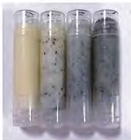
Figure 1. Test material with individual pomace additions of 1, 3, and 5% (including the visible uneven distribution of particles) and the control sample.
