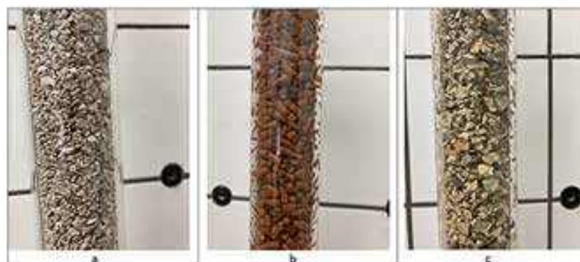
Figure 1. Filtration materials in research columns: (a) modified marl rock opoka (Rockfos®), (b) iron granulate, (c) limestone grit (photo by Walczak)
