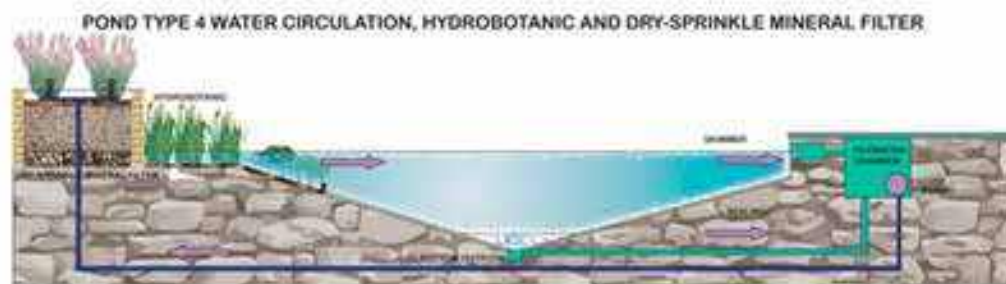
Figure 7. Diagram of the operation of a hydro-botanical swimming pond with accelerated mineral filtration (type 4).
