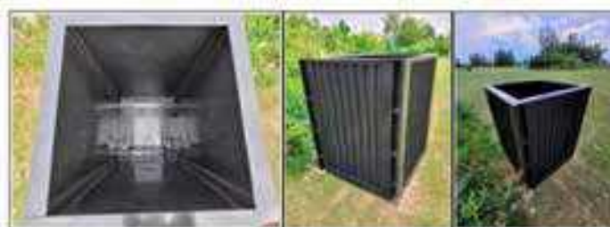
Figure 4. Prototype of a modular filter chamber on a usable scale dedicated to water treatment systems in natural pools (photo: W. Walczak).
