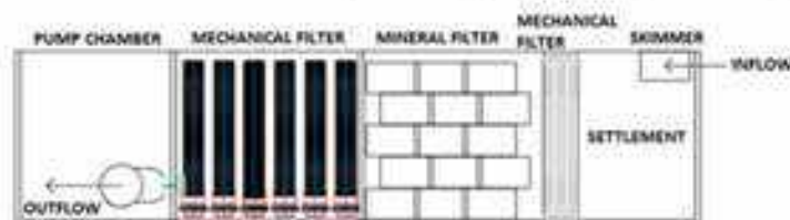
Figure 14. Diagram of the operation of a single-block filter with mechanical and mineral filtration and a suction section.
