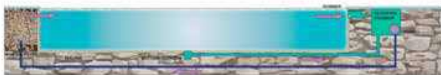
Figure 9. Diagram of the operation of a swimming pond with no regeneration zone (type 5).
