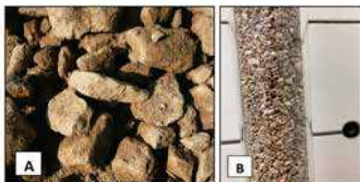
Figure 6. Calcium–silicate rock—opoka. (A) natural material [15], (B) Rockfos ® material (photo: W. Wólczak).
