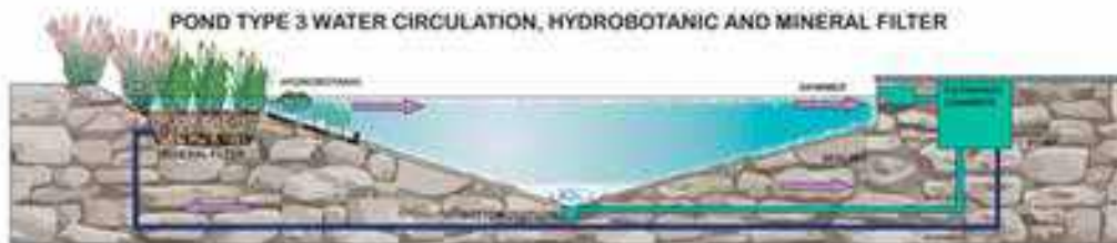
Figure 6. Diagram of the operation of a hydro-botanical swimming pond with a mineral filter (type 3).
