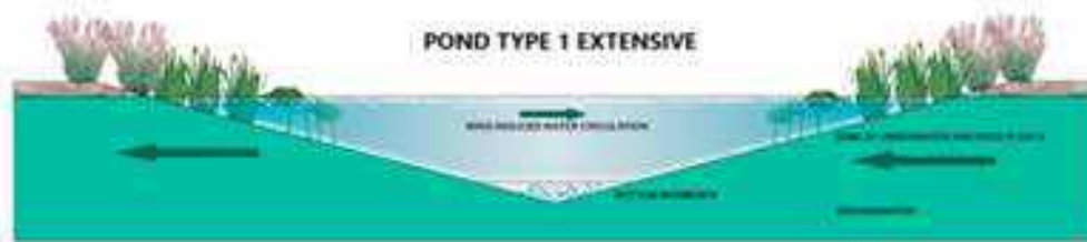
Figure 3. Diagram of the operation of an extensive swimming pond (type 1).
