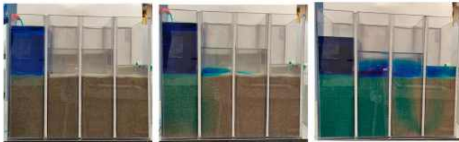
Figure 11. Freeze frames showing the course and position of the flow stream through individual chambers of the model.
