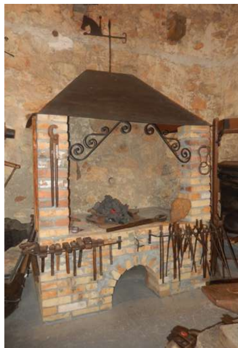
Photo 8.9. The hearth of the blacksmith's furnace in the Wojciechów Blacksmithing Museum. Photo by Anna Mazurek-Kusiak
