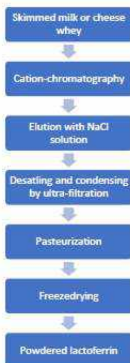
Figure 3. LF production process.
