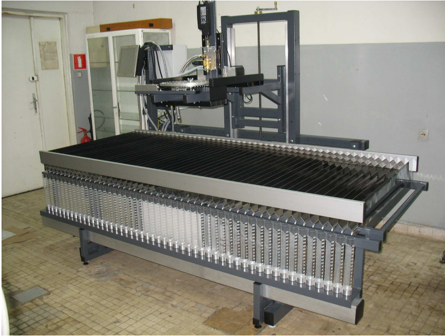
Figure 2. Device for complex measurements of agricultural nozzles
