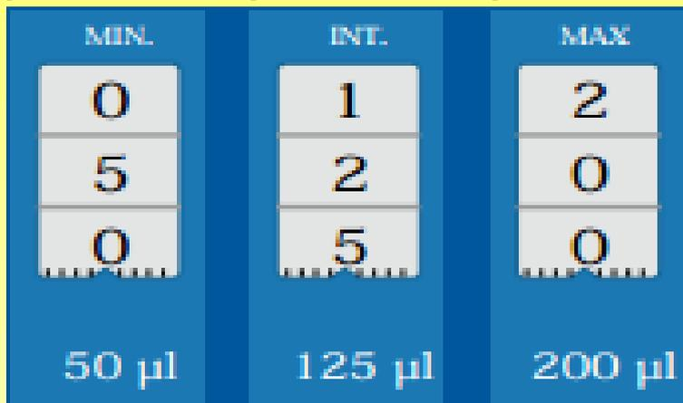
The volume is displayed as three digits which are read from top to bottom. The figure on the left shows the minimum (MIN), intermediate (INT) and maximum (MAX) volume settings.
