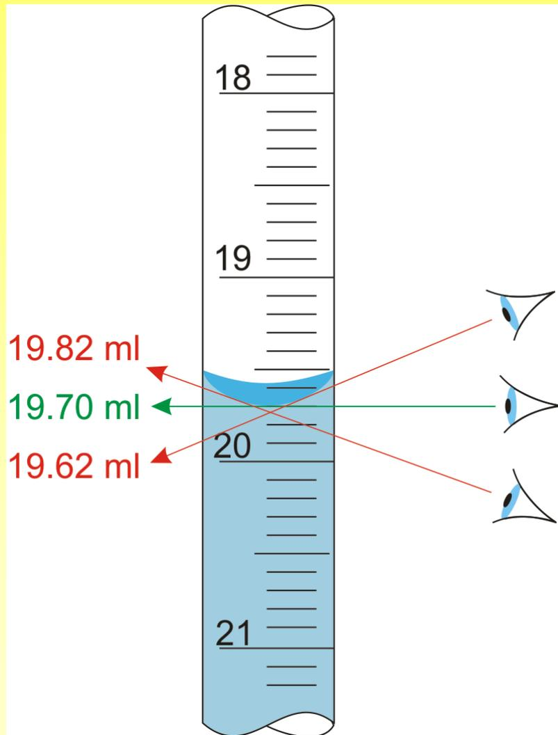
At the time of reading from a pipette or burette eye of the beholder should be at the same level as the liquid, which allows avoid an error.
