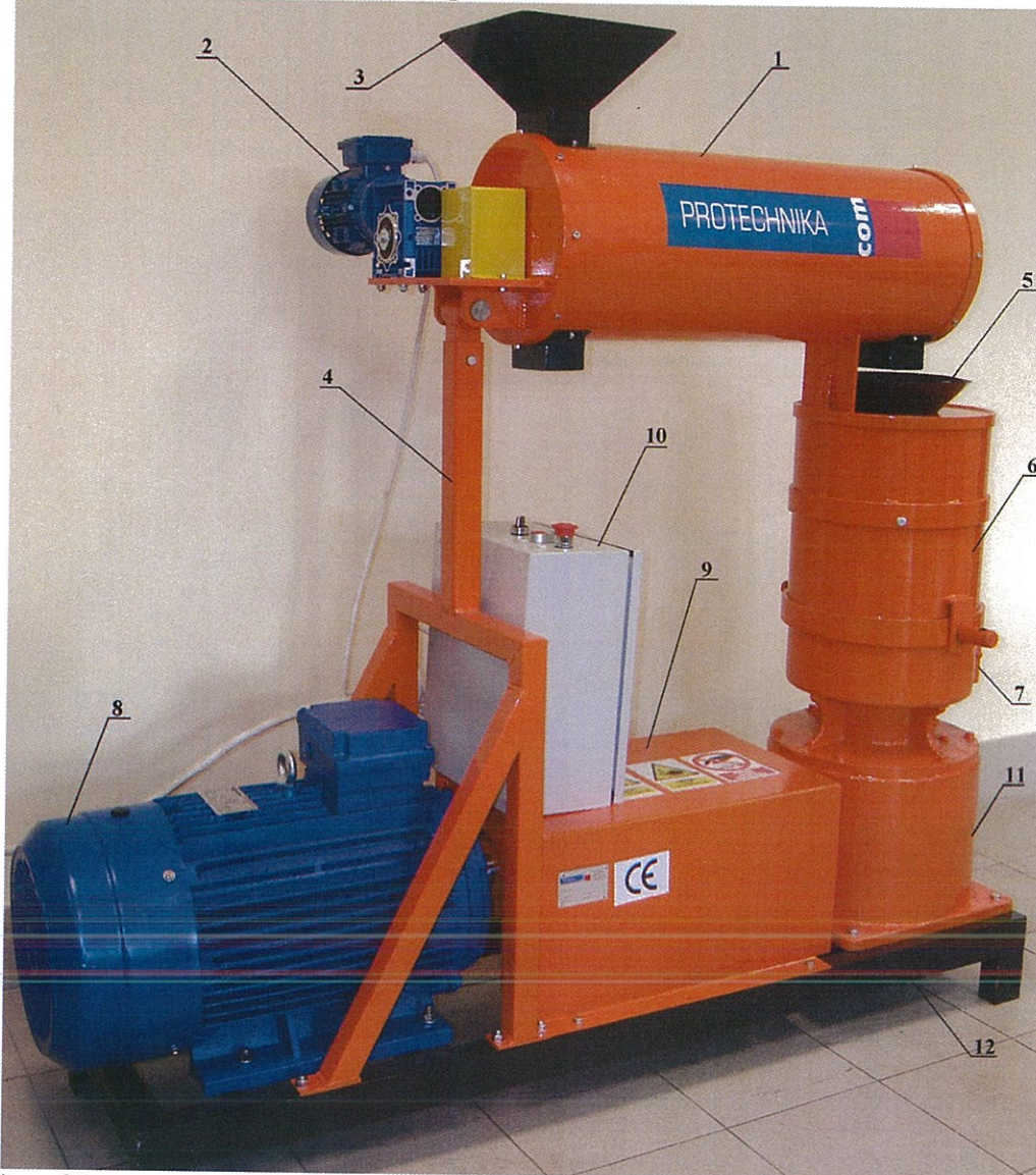
Fig. 1. View of the new pelleting and briquetting device with a flat immovable matrix: 1-mixing/pelleting/dosing system, 2-drive of the mixing/pelleting/dosing system, 3-charger of the mixing/pelleting/dosing system, 4-fixing frame of the mixing/pelleting/dosing system, 5-feeder of material to the working system of the pellet mill, 6-working system of the pellet mill, 7-outlet of pellets from the working system, 8-drive of the pellet mill (electric motor), 9-clutch shield and torque meter, 10-control panel, 11-gear, 12-base
